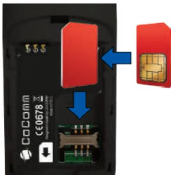
on the terminal match the slots on top of the battery, as shown in the picture. Replace the lid of the battery compartment, ensuring that it is perfectly secured in place.
